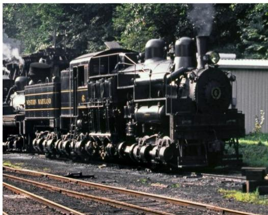
**For the train buff --** The need to transport heavy loads of logs through the mountains required a lot of power. Invented by Ephram Shay, the Shay locomotive was the most widely used geared steam locomotive. The Cass Railroad has the largest roster of Shay locomotives in the world.
