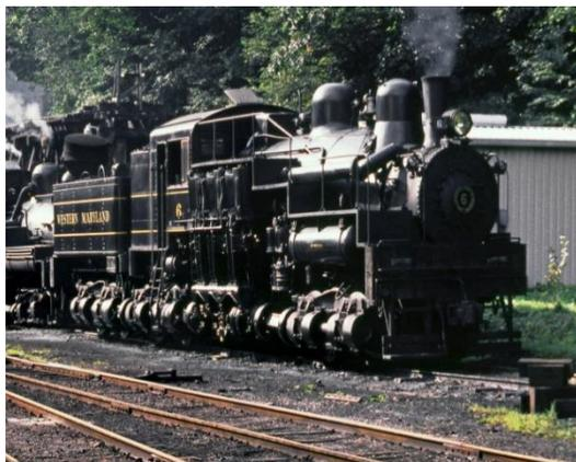
**A note for the train buffs --** The need to transport heavy loads of logs through the mountains required a lot of power. Invented by Ephram Shay, the Shay locomotive was the most widely used geared steam locomotive. The Cass Railroad has the largest roster of Shay locomotives in the world.
